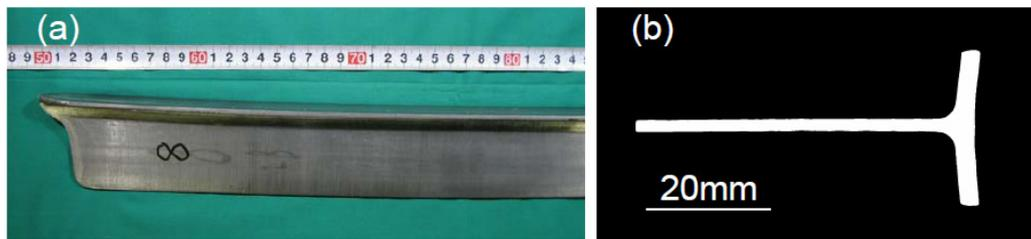
Fig. 9. Pure lead T-bar rolled with new facilities: (a) appearance of top end, (b) cross section at center of length.
