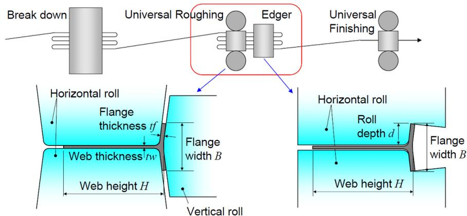
Fig. 1. Mill layout of T-bar rolling and schematic diagrams of Universal Roughing and Edger rolling.
