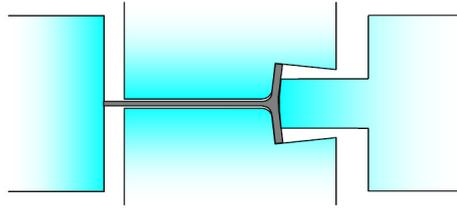
Fig. 8. Arrangement of new edger with vertical rolls.
