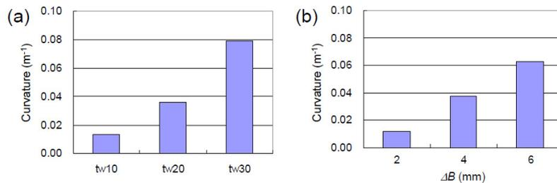
Fig. 4. Curvatures of side camber by FE simulation: (a) three sections of universal rolling, (b) three edger rolling conditions.
