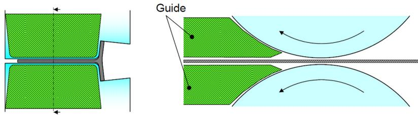
Fig. 5. Geometry and position of guide.
