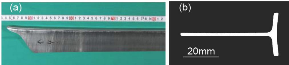
Fig. 7. Rolled pure lead T-bar: (a) appearance of top end, (b) cross section at center of length.
