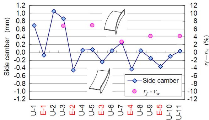
Fig. 6. Side camber and thickness reduction difference.
