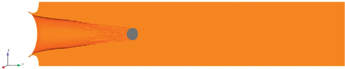
Figure 3. Steel sphere penetration into semi-infinite adobe target ( V_0 = 1200 m/s). (Note that penetration depth results from 2-D CTH simulations only are reported in this paper. A three-dimensional simulation image is shown here because it better illustrates the plastic deformation of the sphere, which is more difficult to visualize from the 2-D results.)
