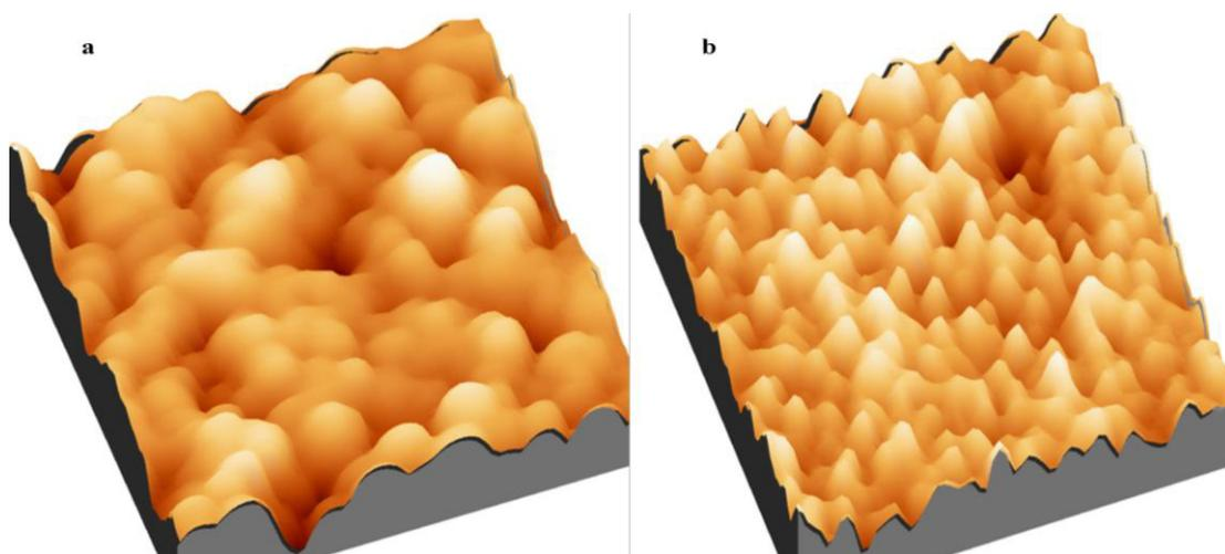
Fig. 3 (a) AFM image of BMO/Si (100) film; (b) AFM image of BMO/Si (111) film
