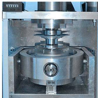
Fig. 7: Ring-on-Disc test plant with mounted pair of specimen [EndoLab (2015)]
