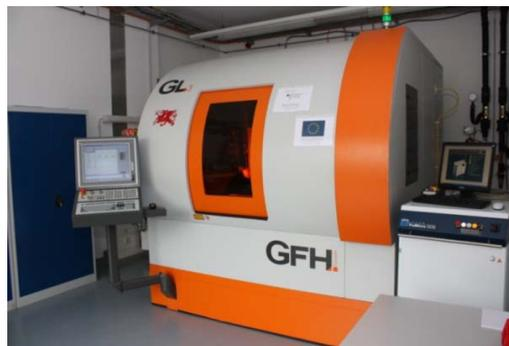
Fig. 1: USP-micromachining system at the SLV M-V GmbH
