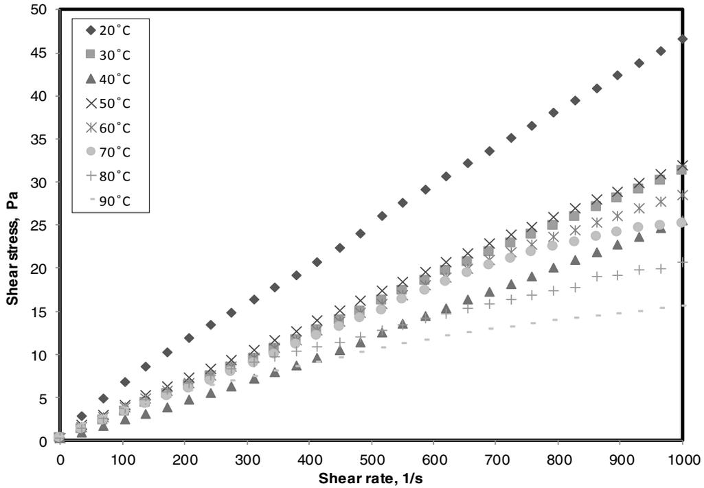
Fig. 1. Shear stress versus shear rate at 40% volume water fraction
