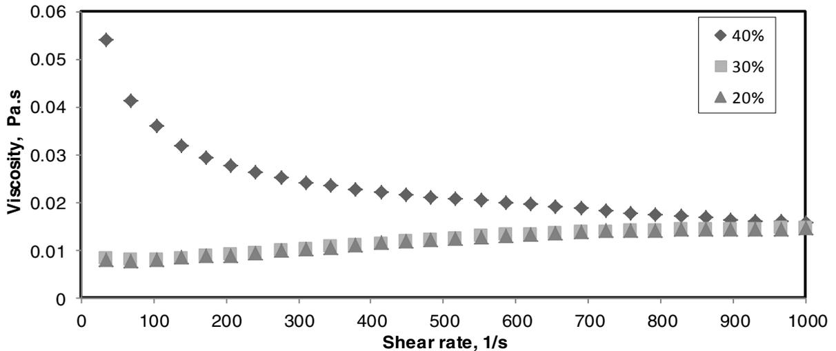
Fig. 3. Effect of water volume fraction on viscosity at  $90^\circ\text{C}$
