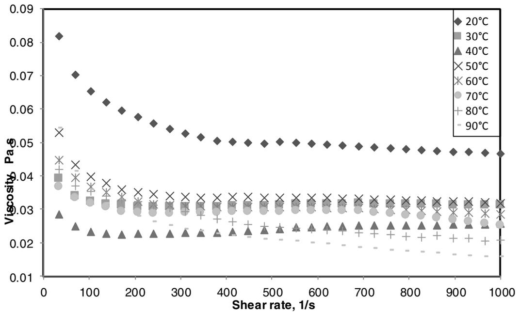
Fig. 2. Effect of temperature on viscosity at 40% water fraction
