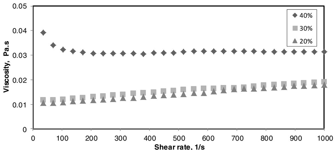
Fig. 4. Effect of water volume fraction on viscosity at 30°C
