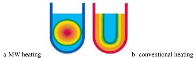
Fig. 1. Microwave heating and conventional heat dissipation
