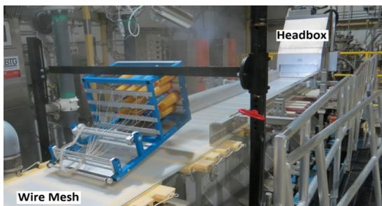
Fig. 4. Installed feeding frame on the paper machine table
