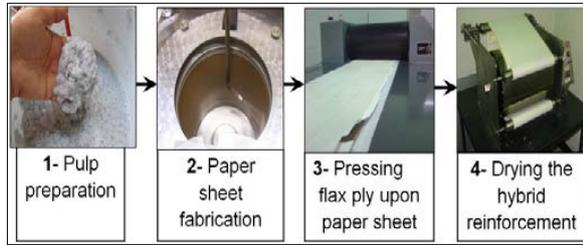
Fig. 7. Processing of the reinforcement in laboratory
