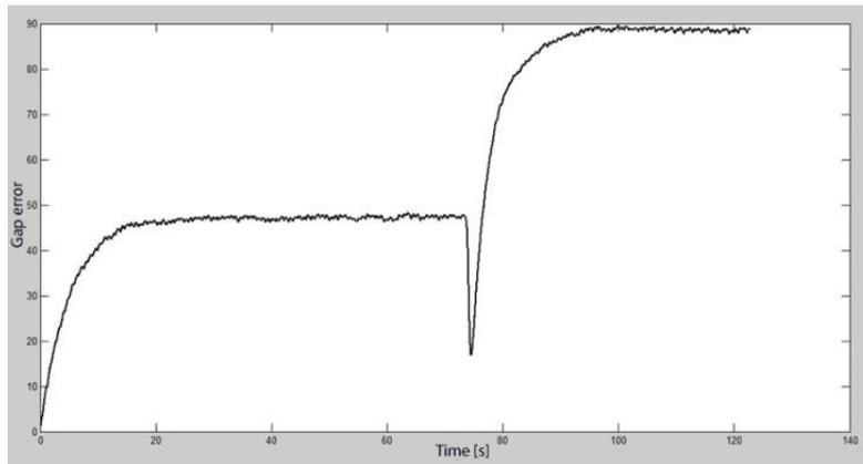
Fig. 4. Gap error vs Time in a test with 40-20mm thickness variation workpiece.
