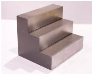
Fig. 1. Workpiece used for the variable characterization, with 60–40–20mm thickness variation.
