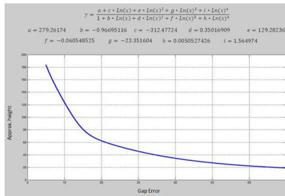
Fig. 6. Thickness determination curve in a workpiece with 40-20mm thickness variation.
