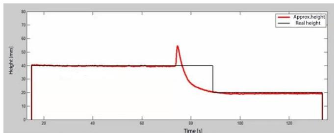
Fig. 7. Offline thickness determination curve in a workpiece with a 40-20mm thickness variation.
