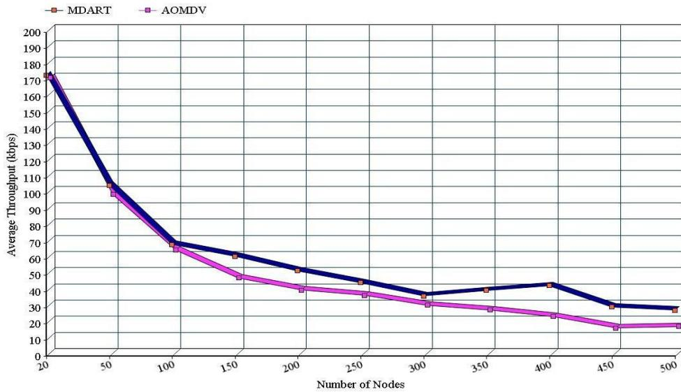
Fig.4: Average Throughput Comparison of MDART and AOMDV
