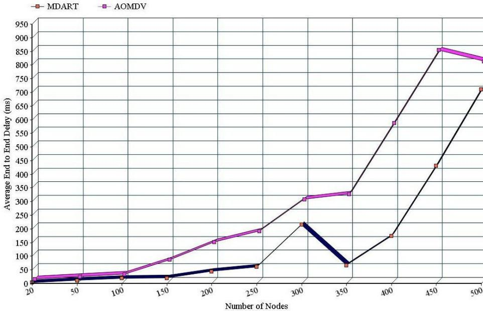
Fig.6: Average End to End Delay comparison of MDART and AOMDV
