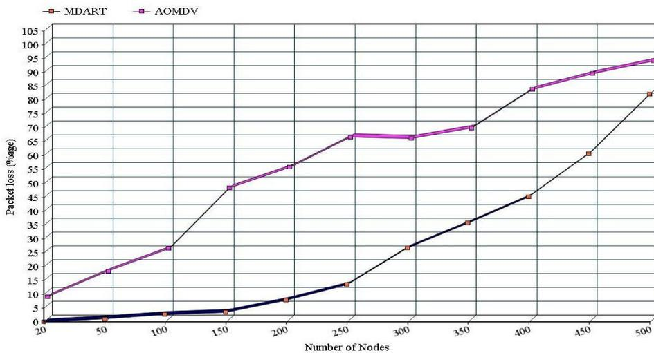
Fig.5: Average Packet Loss Percentage Comparison of MDART and AOMDV
