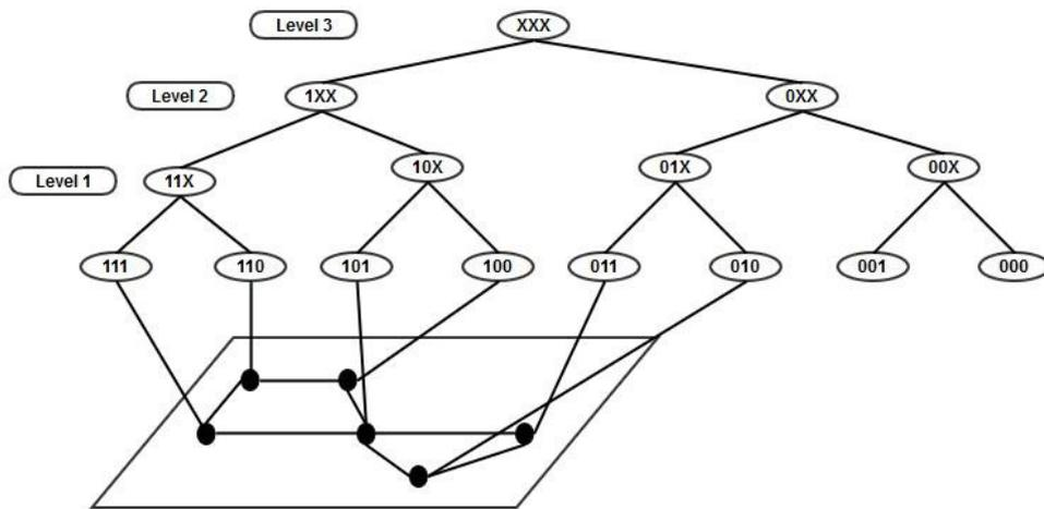
Fig.3: Representation of Address space overlay upon the basic physical topology of network
